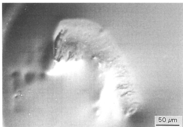
Figure 7 Environmental electron micrograph of a fracture surface for an interfacially modified crumb rubber–asphalt system.
